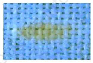
**Figure 5a.** Ultraviolet induced blue fluorescence of linen after irradiation with ArF laser in the working point of the third row of table 1. The irradiated area is recognized by the lack of fluorescence. From Ref. [24].
