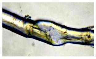
**Figure 3**. Microscope image of a single linen fiber colored with ArF laser. The mechanical damage in the middle shows a colorless inner medulla. Contrast-enhanced detail of figure 8 in Ref. [24].
