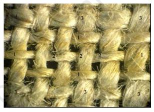
**Figure 2**. The linen area irradiated by ArF laser pulses shows different characteristics corresponding to the local laser intensity value I(x,y). 1) colored area; 2) ablated area; 3) area irradiated below threshold for coloration. From Ref. [24].
