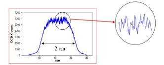
**Figure 7.** Two-dimensional intensity shape of the laser beam measured by a CCD camera Andor model DV-430UV, having a single pixel resolution 11  $\mu$ m = 0.011 cm. The inset shows a zoom of the high-frequency intensity fluctuations.
