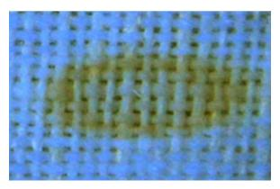
**Figure 5b.** Ultraviolet induced blue fluorescence of linen after irradiation with ArF laser in the working point of the seventh row of table 1. In this case, the lack of fluorescence is not uniform across the laser irradiated region.
